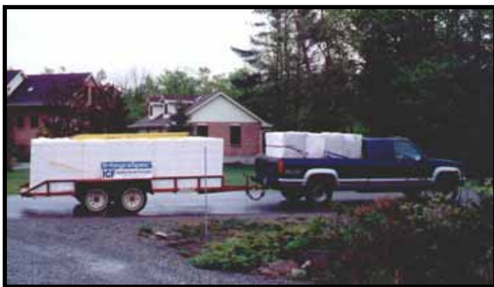
Shown: Shipment for 1200 ft 2 foundation, eight units high
