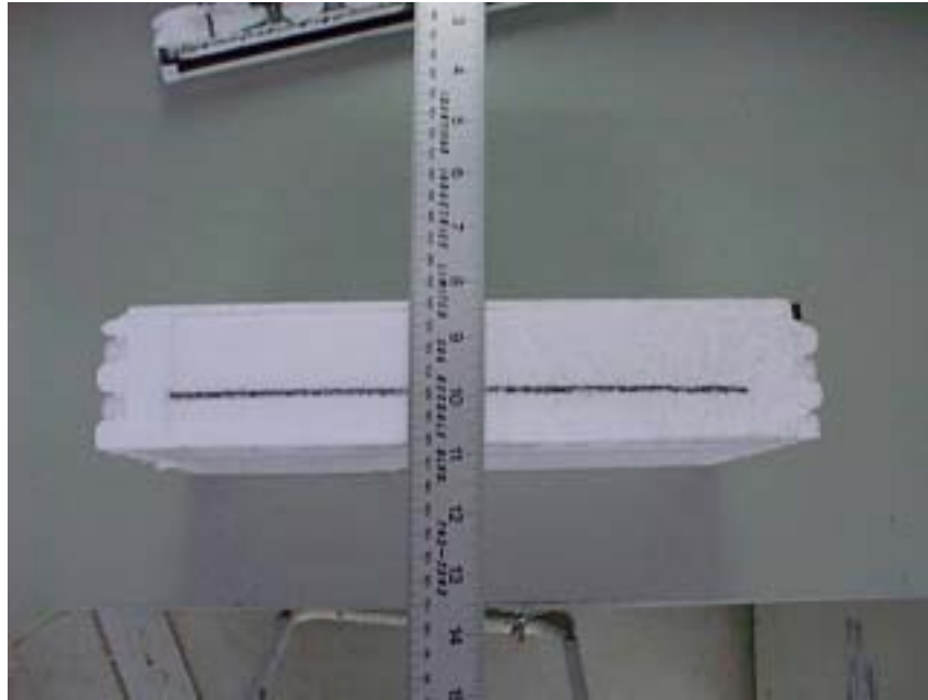
Photograph no. 3: Cut edge of plastic foam insulation showing position of the polystyrene channel face.
