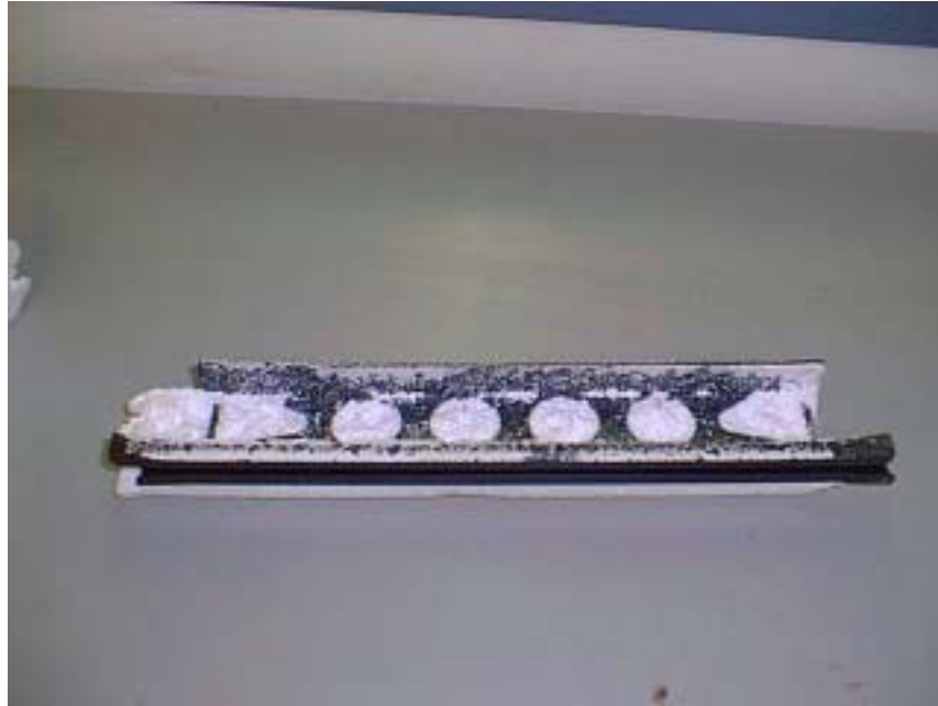
Photograph no. 1 : Typical test specimen of polystyrene channel.
