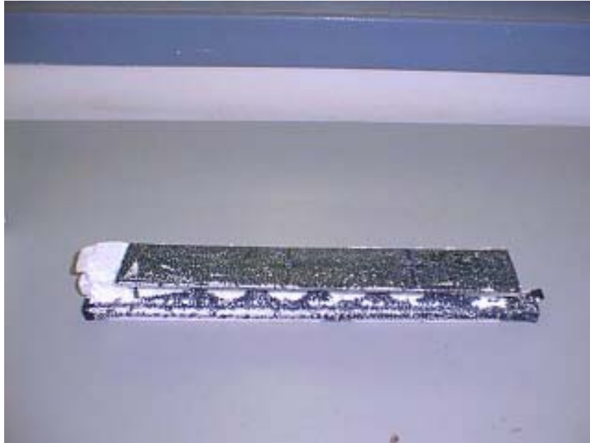
Photograph no. 2 : Typical tested specimen of polystyrene channel showing positions of the screws.
