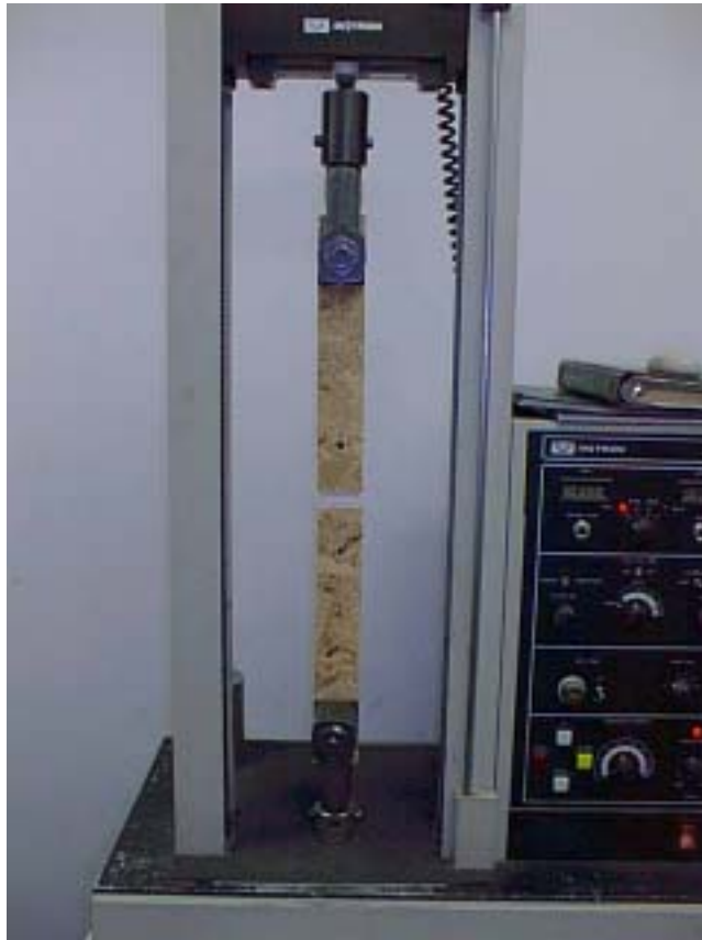
Photograph no. 5: Test set-up for lateral screw resistance tests.
