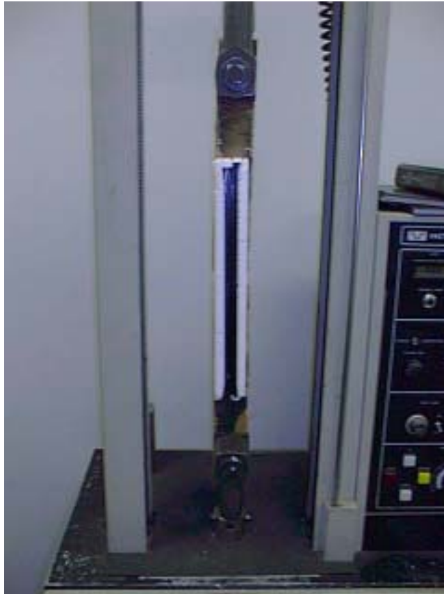
Photograph no. 6: Test set-up for lateral screw resistance tests.
