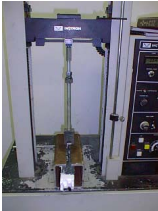
Photograph no. 4: Test set-up for screw withdrawal tests, showing fixtures used to support the specimens and grip the screws.
